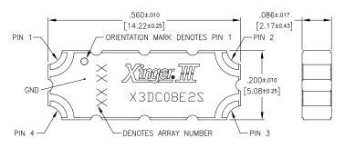
Dimensions are in Inches [Millimeters] X3DC08E2S Mechanical Outline
